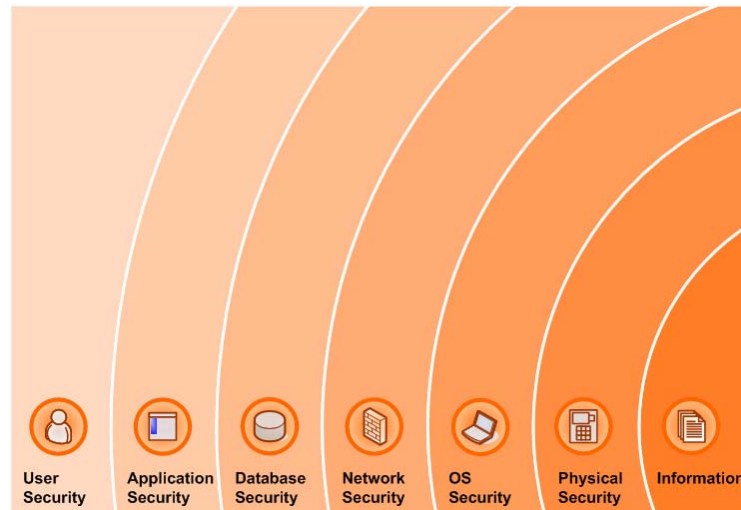
Figure 6 –Defence in Depth: A Layered Approach
