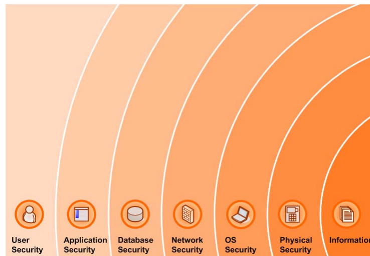
Figure 4—Defence in Depth: A Layered Approach
